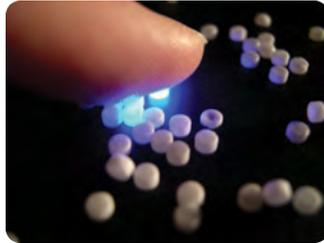
Plasma-shells™ are hollow gas encapsulating devices developed by Imaging Systems Technology (IST). When a voltage is applied across the walls of the shell, the encapsulated gas is energized into plasma. The Plasma-shells™ are electronic components that can be used as light emitters, switches, and sensors. Under a sister company, Deep Springs Technology (DST), hollow shells are being introduced into mechanical and structural applications including armor, buoyancy, and heat shielding.
